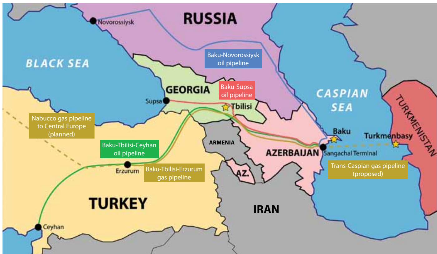
This map shows the existing and planned oil and gas pipelines from Baku, Azerbaijan, including the Baku-Tbilisi-Erzurum pipeline.
